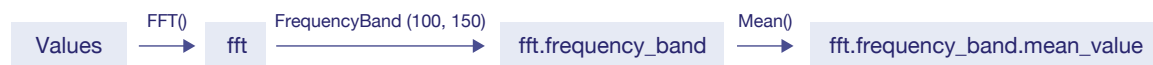
Figure 3-6: An example feature produced by applying the FFT and FrequencyBand transformations, followed by the Mean aggregation, to the input array values.
